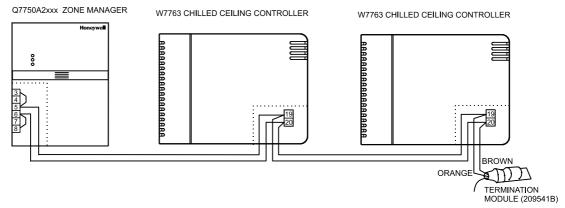
Note: C7750A Zone Manager has internal termination module (with jumpers installed as shown).
