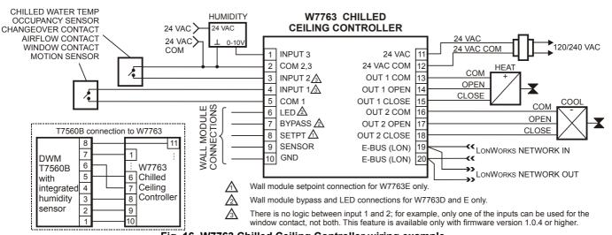
Fig. 16. W7763 Chilled Ceiling Controller wiring example
