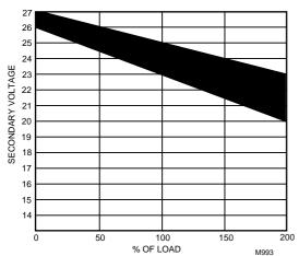
Fig. 13 NEMA class 2 transformer voltage output limits
