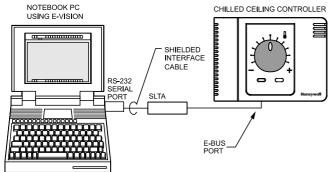
Fig. 9. Connecting the portable operator terminal to LonWorks Bus
