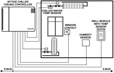
Fig. 2. Typical W7763 Chilled Ceiling control application
