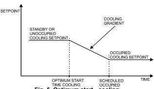
Fig. 5. Optimum start - cooling
