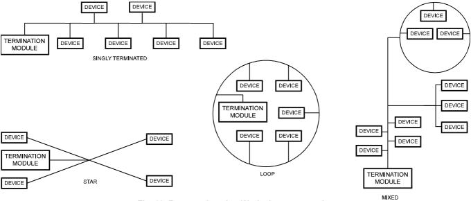
Fig. 12. Free topology LonWorks layout examples
