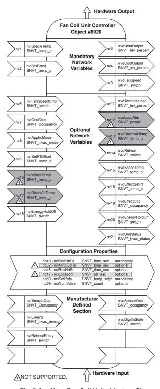
Fig. 7. LonMark Fan Coil Unit object profile
