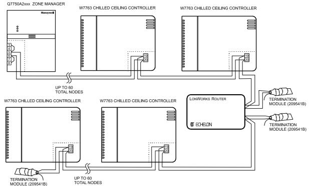
Fig. 11. LonWorks Bus wiring layout for two daisy-chain network segments
